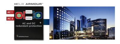
**AC assurance** - HELIX AC utilizes and monitors two ac branch circuits. Trouble to a primary branch instantly switches power to the back up branch to maintain uninterrupted system operation.
